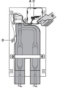
4 Use a small screwdriver and follow indicated instructions for connecting cable wires into the terminal connector according to the wiring diagram.
